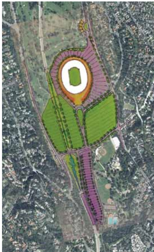
Reorganization of the parking around the Rose Bowl could include a realignment of the stadium entry road to allow more efficient use of adjoining spaces; impervious parking surfaces with reinforced turf to support parking, recreation, and stormwater harvesting; and improved parking flow and striping layouts to maximize use on large event days.
